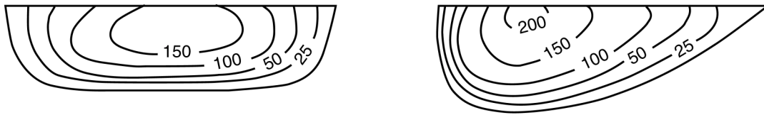
Figure 19.1—Idealized diagrams of the patterns of flow in cross-section of open channels: left shows the pattern on a straight reach, right shows the pattern on a bend. The units on the lines of equal flow-rate could be centimeters per second. (modified from Hynes 1970)
