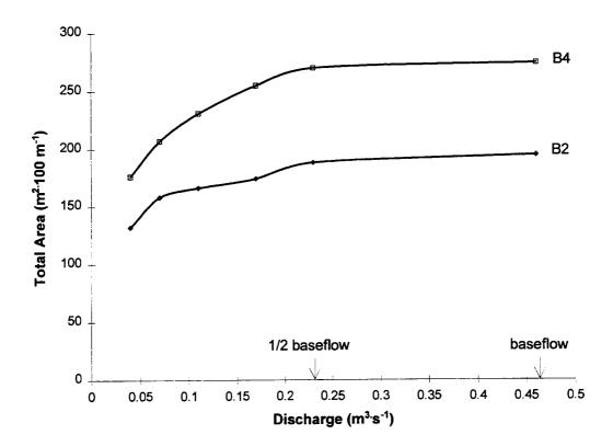
Figure 5. Total area  $(m^2\cdot 100~m^{-1})$  as a function of discharge  $(m^3\cdot s^{-1})$  for reaches B2 and B4 in Hunt Creek.
