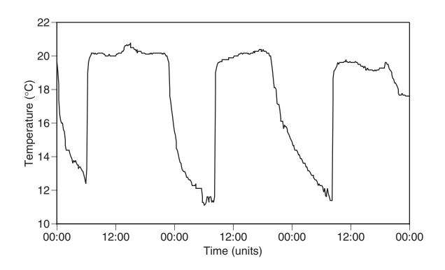
Figure 9.–Temperature patterns at Alcona peaking project on the Au Sable River, Michigan.
