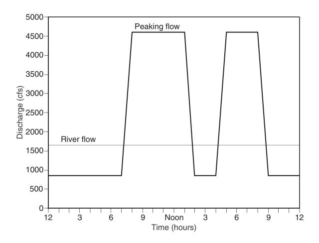
Figure 8.–Typical daily peaking flow pattern at Tippy Dam.
