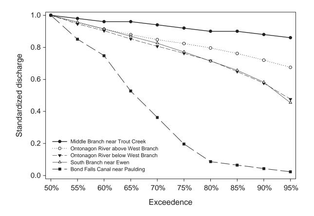
Figure 13.–Standardized low-flow duration curves for sites in the Ontonagon River watershed that are affected by the Bond Falls diversion. Data from United States Geological Survey gauge stations. Period of record was 1942–71 for the South Branch and 1942–2004 for the other four sites.
