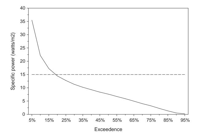
Figure 39.–Specific power for the West Branch Ontonagon River near Bergland.
