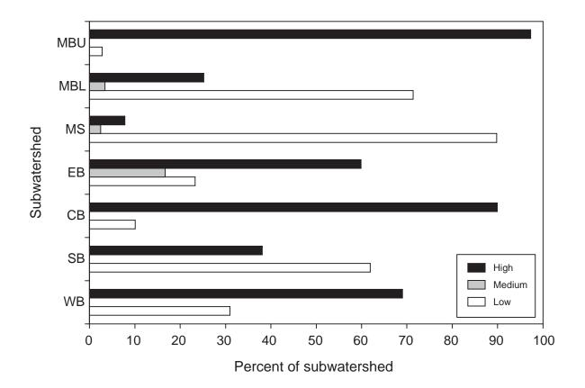
Figure 5.–Composition of surficial deposits within the seven subwatersheds of the Ontonagon River basin. High, medium, and low refer to the permeability of the surficial material. Subwatershed codes: MBU = upper Middle Branch, MBL = lower Middle Branch, MS = Main Stem, EB = East Branch, CB = Cisco Branch, SB = South Branch, and WB = West Branch.
