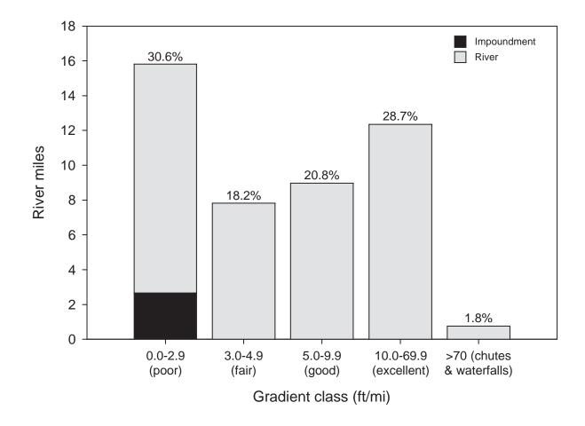
Figure 22.–Stream gradient distribution for the Middle Branch Ontonagon River from the origin at Crooked Lake to Agate Falls. Fish habitat ranking in parentheses.
