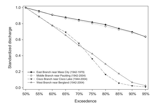
Figure 11.–Standardized low-flow duration curves for sites in the Ontonagon River watershed that are not affected by the Bond Falls diversion. Data from United States Geological Survey gauge stations for period of record.
