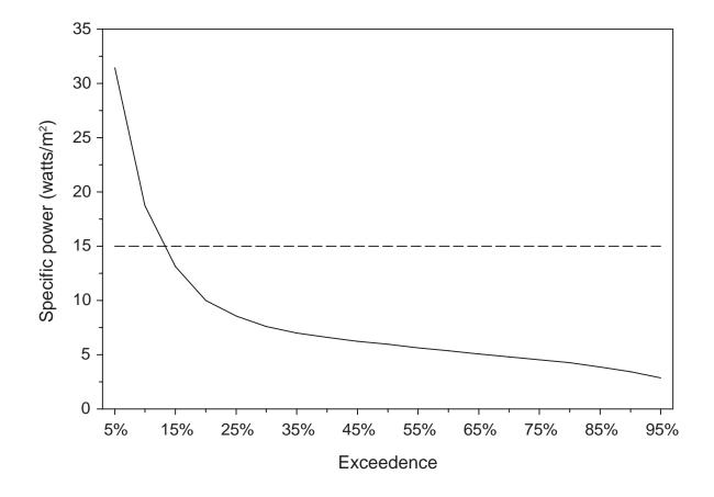
Figure 28.–Specific power for the main stem Ontonagon River downstream of the confluence with the West Branch.
