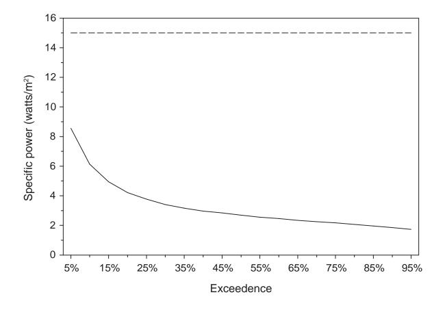
Figure 23.–Specific power for the Middle Branch Ontonagon River near Paulding.
