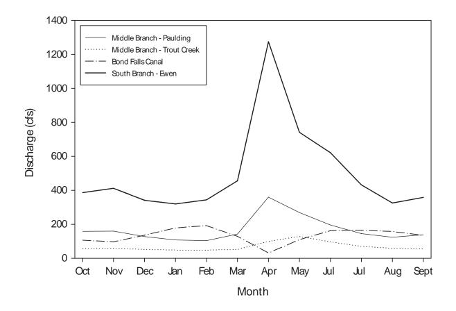
Figure 10.–Mean monthly discharge at United States Geological Survey gauge sites on the Middle Branch Ontonagon River (Middle Branch – Paulding [above Bond Falls] and Middle Branch – Trout Creek [below Bond Falls]), the Bond Falls Canal, and the South Branch Ontonagon River. The period of record was 1942–71 for the South Branch and 1942–2004 for the other three sites. Note that less water was diverted through the Bond Falls Canal during April, the time of peak discharge in the South Branch.
