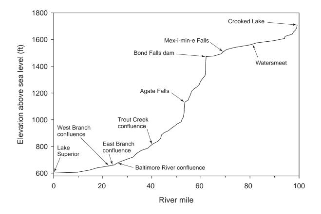
Figure 21.–Elevation changes by river mile for the Middle Branch and main stem Ontonagon rivers.
