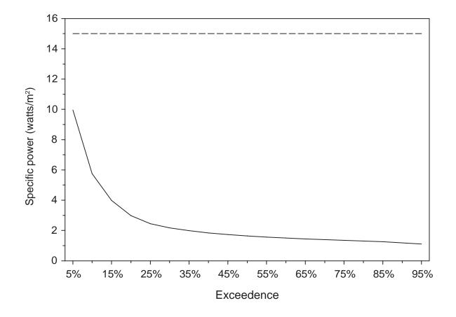
Figure 27.–Specific power for the main stem Ontonagon River upstream of the confluence with the West Branch.
