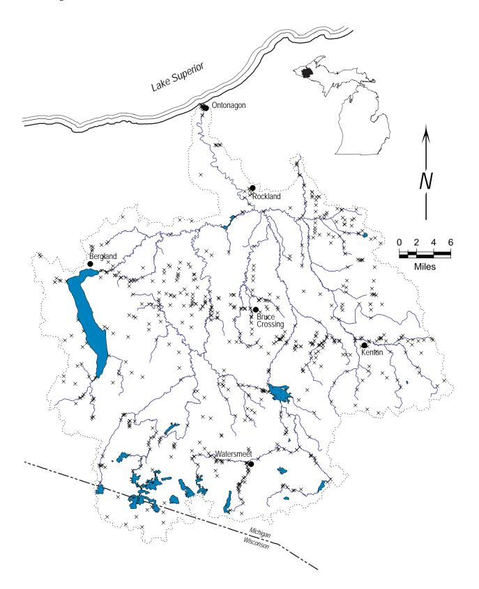
Figure 20.–Stream crossings in the Ontonagon River watershed (includes roads, railroads, and utilities). Stream crossing data derived from MIRIS Base Data (1998).
