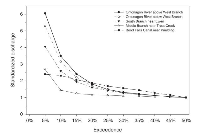
Figure 14.–Standardized high-flow duration curves for sites in the Ontonagon River watershed that are affected by the Bond Falls diversion. Data from United States Geological Survey gauge stations. Period of record was 1942–71 for the South Branch and 1942–2004 for the other four sites.
