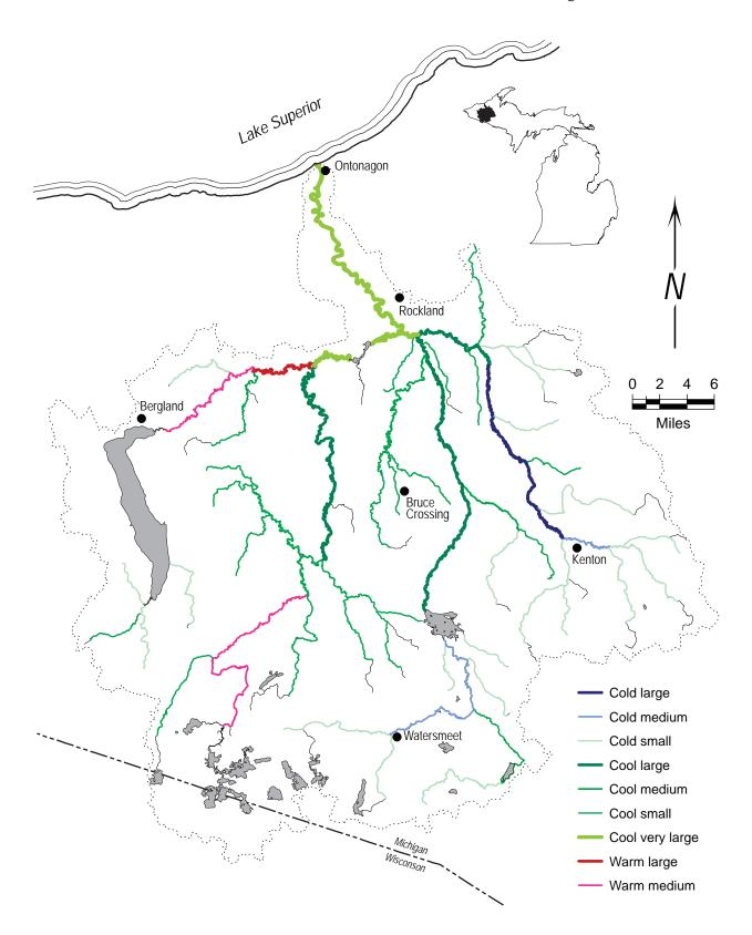
Figure 43.–Valley segments of the Ontonagon River watershed classified by stream temperature and catchment area (Baker 2006). Mean stream temperature during the first three weeks of July:  $cold = <66^{\circ}F$ ,  $cool = 66-72^{\circ}F$ , and  $warm = >72^{\circ}F$ ; catchment area at the midpoint of the segment: small (headwater) = 10–40 mi<sup>2</sup>, medium = 40–179 mi<sup>2</sup>, large = 180–620 mi<sup>2</sup>, and very large = >620 mi<sup>2</sup>.
