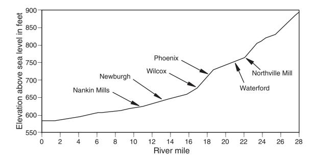
Figure 28b.–Elevation changes, by river mile, from the headwaters to the mouth, of the Middle Rouge River. Major mainstem dam locations are shown. Data from: Knutilla, 1970.
