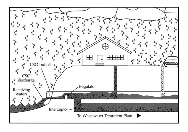
Figure 32.–Illustration of a typical combined sewer system. CSO = combined sewer overflow. Prepared by: Southeast Michigan Council of Governments.
