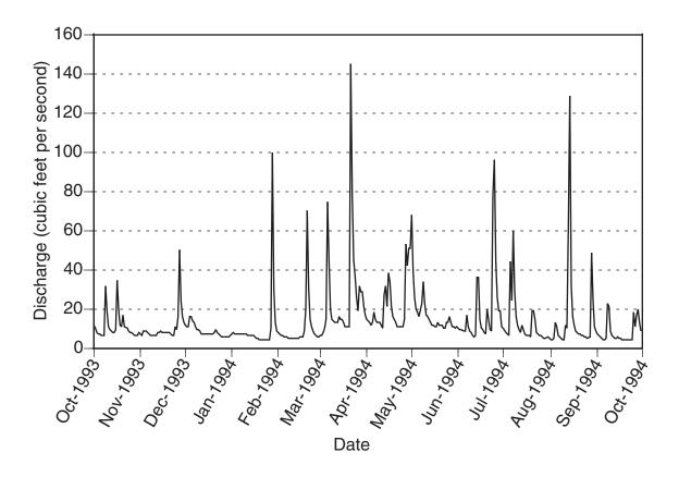
Figure 13.—Mean daily discharge of Upper Rouge River in Farmington for water year 1994. Data from: United States Geological Survey.
