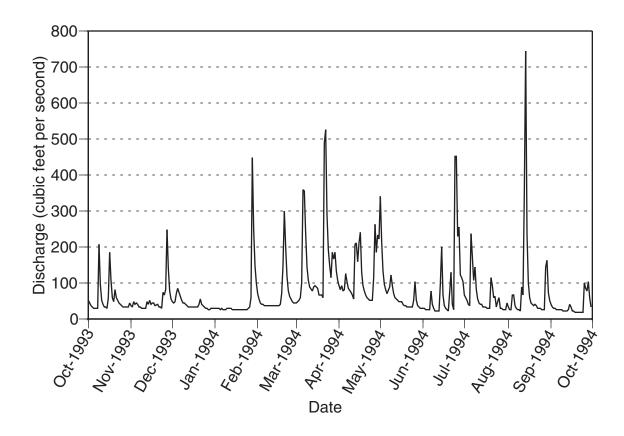
Figure 14.—Mean daily discharge of Middle Rouge River near Garden City for water year 1994. Data from: United States Geological Survey.
