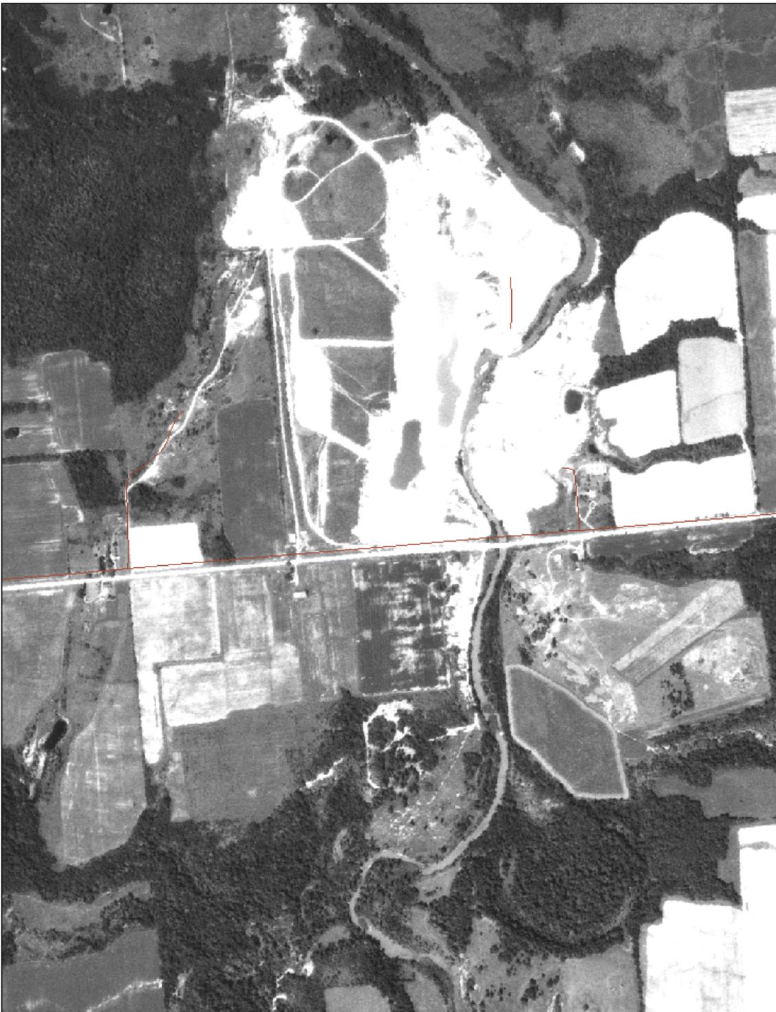
Fifth of eight aerial photos of the Black River at Fisher Rd. The mining operation has expanded with modifications apparent in the river channel in September, 1980.
