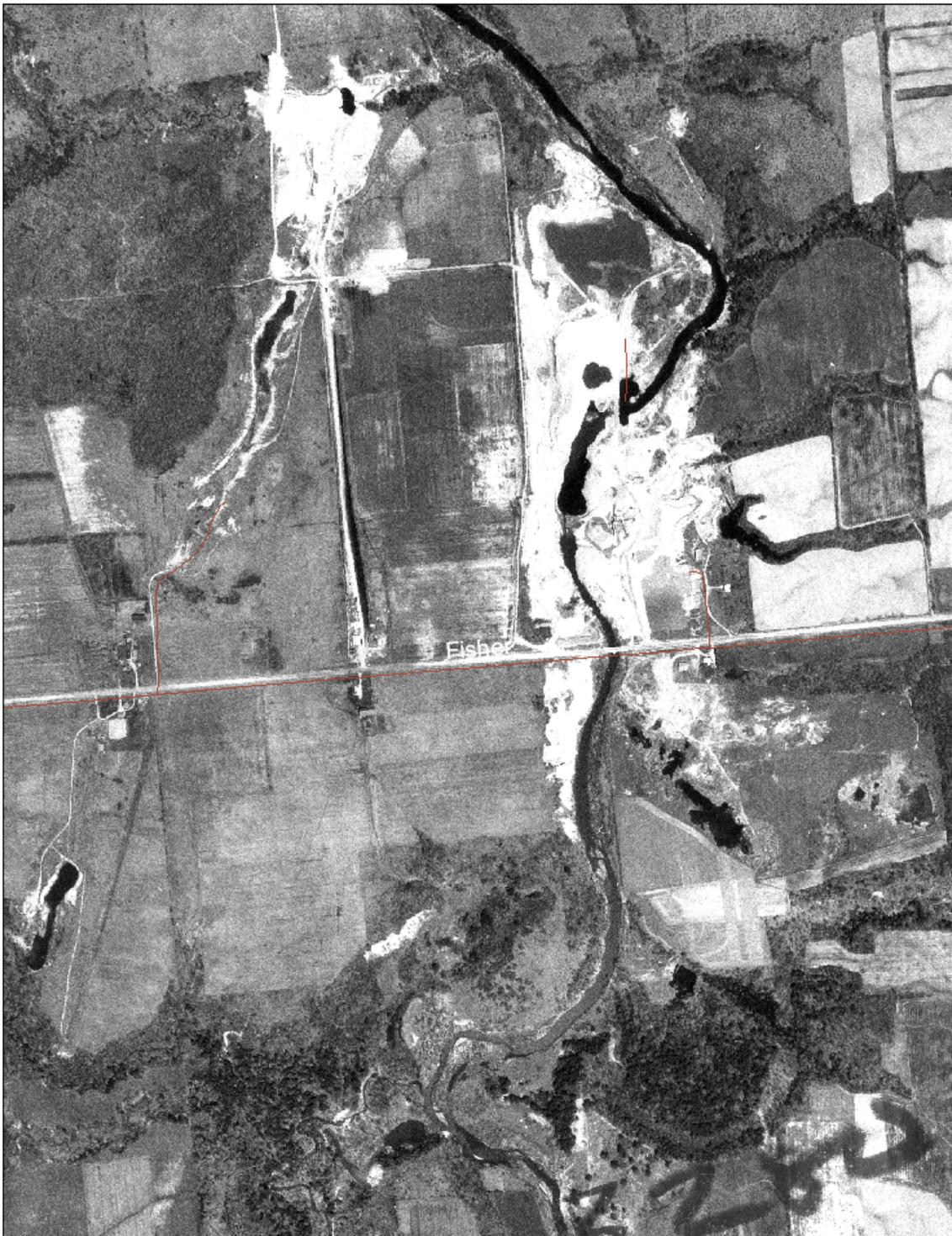
Fourth of eight aerial photos of the Black River at Fisher Rd. A mining operation is apparent with heavy silt loading into the river in May, 1971.
