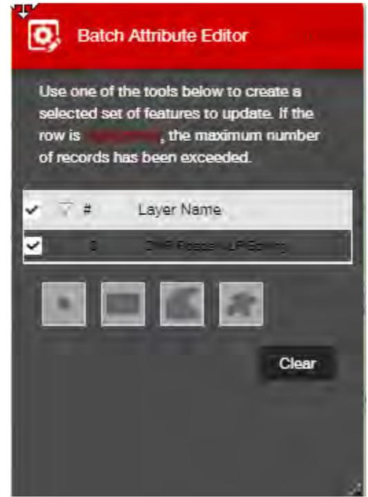
The Batch Editor is used for selecting multiple road segments and batch changing an attribute.
