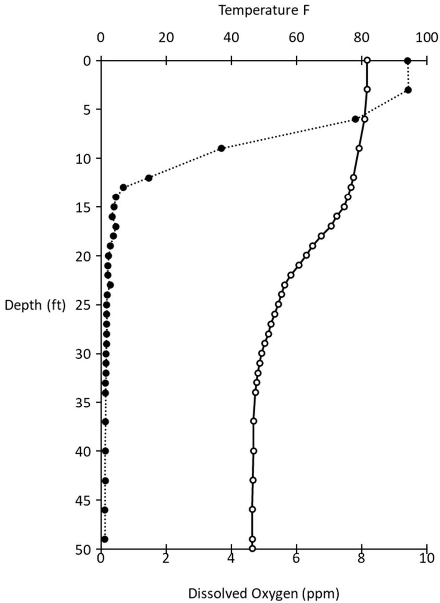
Figure 1. Temperature and dissolved oxygen profile of Long Lake recorded August 11, 2016. The solid line with open circles represents temperature. The dotted line with black circles represents dissolved oxygen.
