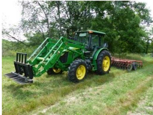
Tractor equipped with HedgeHog bar for removal of invasive shrubs.
