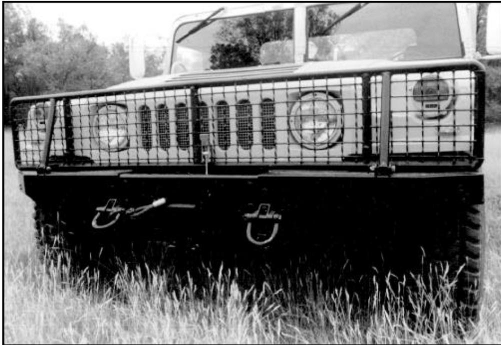
**Figure 10** – Bumper extensions and a folding grill guard.
