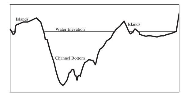
Figure 13b.-Aggraded mainstem channel-cross section below Tippy Dam.
