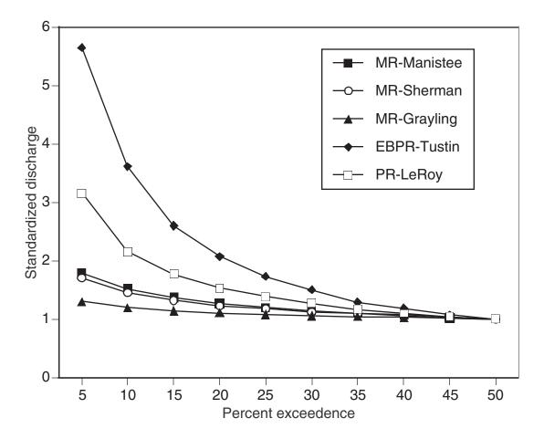
Figure 6.–Flow duration curves for selected sites on the Manistee and Pine Rivers. Information from United States Geological Survey for period of record.
