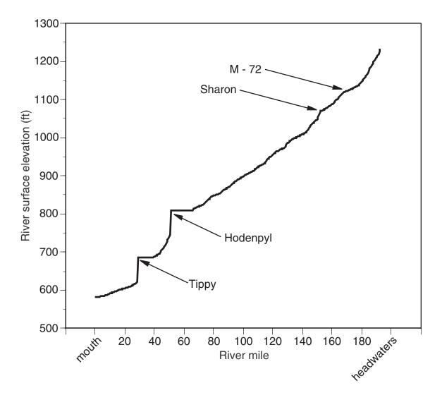
Figure 10.-Gradient (elevation change in ft/mi) of the Manistee River.
