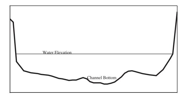
Figure 13a.-Degraded mainstem channel-cross section below Tippy Dam.
