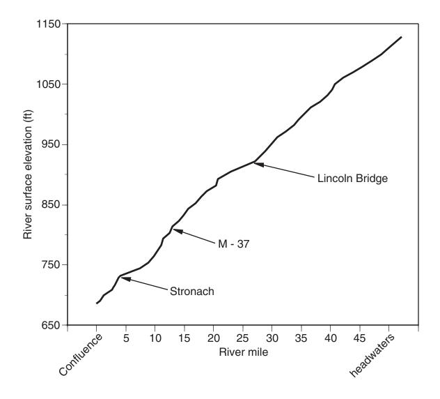
Figure 11.—Gradient (elevation change in ft/mi) of the Pine River.
