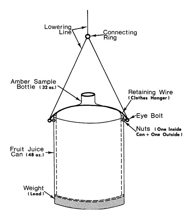
Figure 2.4–Phytoplankton (chlorophyll) sampler construction plans.
