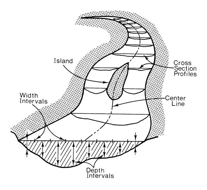
Figure 2.3–A stream sample station showing morphology measurements of length, widths, depths, and cross-section profiles.
