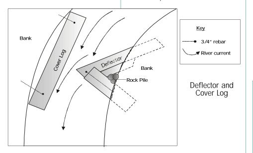
should always be placed nearly parallel to water flow. Placing the tree perpendicular may cause erosion around the ends.
