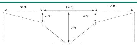
Example of a deep water pond with minimal shallow edges, due to a 3:1slope reaching 4 ft deep, a deep water level of 12 ft.to facilitate a diversity of fish species, and a 25% open water area,24 ft.across, which provides the correct temperatures and amounts of dissolved oxygen, depending on the season.
