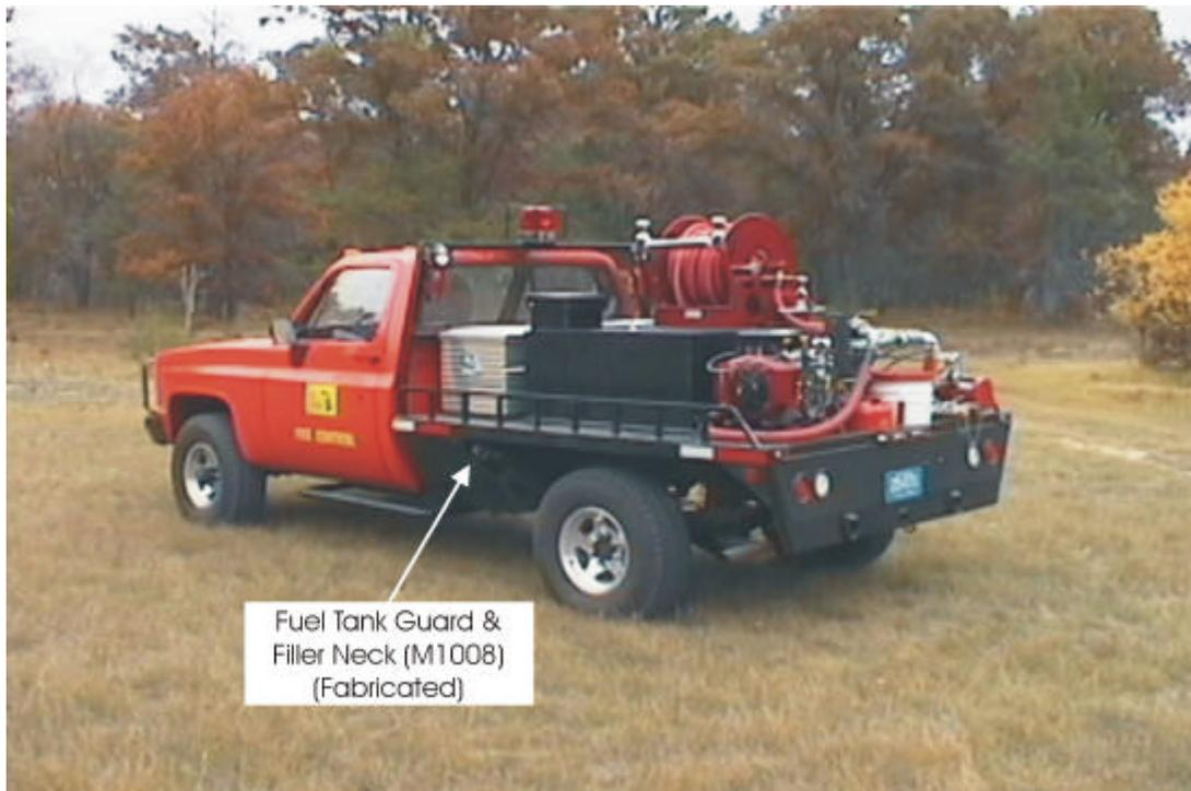
The M1008 has an outside the frame fuel tank which should be guarded.
