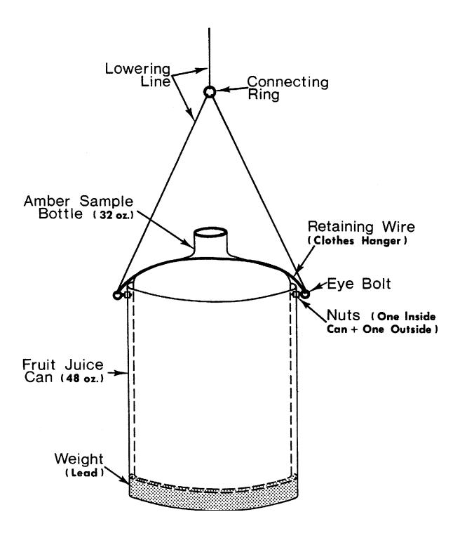
Figure 2.4–Phytoplankton (chlorophyll) sampler construction plans.
