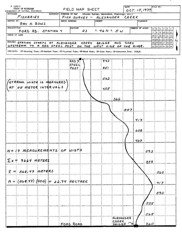
Figure 2.2–Example of use of Field Map Sheet to indicate length, width, area, and orientation of stream study station.
