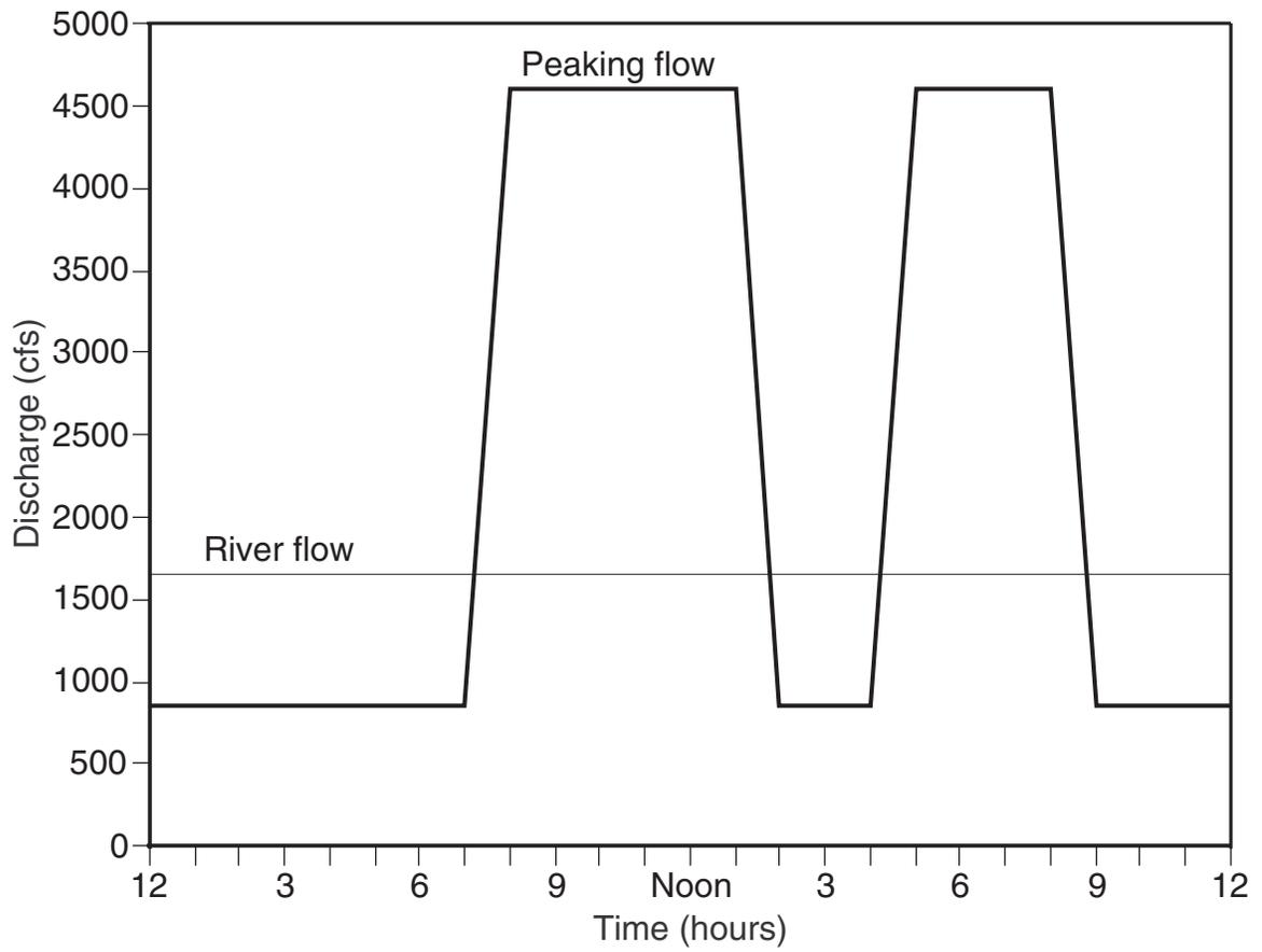
Figure 8.-Typical daily peaking flow pattern at Tippy Dam.
