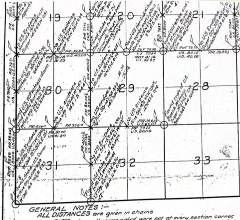
IRON PIPES unless otherwise noted, were set at every section corner, quarter and eighth post, for which witnesses appear on this map. A 3 xxx wooden stake was also set. The center of the Iron pipe is the corner location. No corners were corrected without setting Irons, unless otherwinded hereon."
