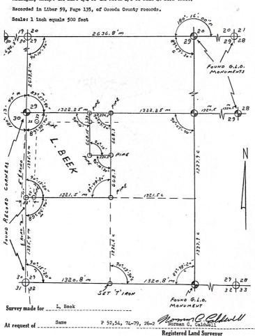
I, NORMAN C, CALDWELL, Registered Land Surveyor, hereby certify that I have surveyed the following described percel of land in accordance with Act 132, P. A. 1970, that the ratio of misclosure is less than 1 part in 5000, and that such is within the present acceptable limits:
