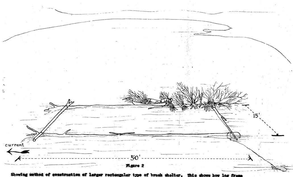
Showing method of construction of larger rectangular type of brush shelter. This shows how log frame is made in position, and how brush is attached — either shole bushes, snage or fagots of small brush. After the brush is added, the shelter is sunk using pairs of sand bags.
