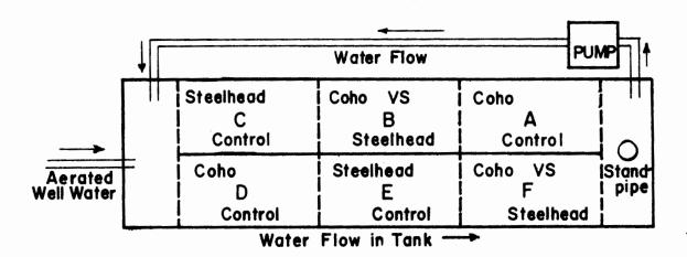
Figure 1. --Diagram of recirculating system in tank with assigned compartments.
