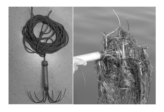
Figure 4.—Photographs of hook designed and constructed to sample submerged plants in Lake St. Clair. Hook was constructed from iron pipe filled with lead and armed with eight tines of steel drill rod.
