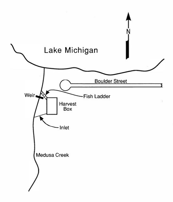
Figure 1. Location and schematic diagram of the Medusa Creek weir complex.
