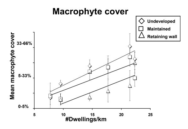
Figure 8.–Macrophyte cover for three different shoreline modifications in six study lakes. Survey sites were 40m long and conducted parallel to shore, at the 0.5m depth contour.
