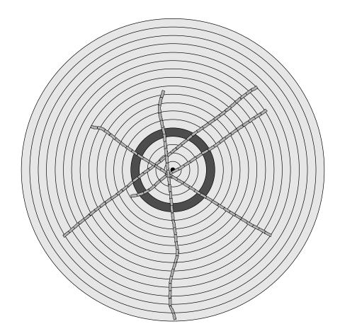
Figure 3.–Illustration of donut polygons used to estimate lake sturgeon abundance from sidescan sonar images for a selected area in Lake St. Clair. Sidescan sonar tracks, each composed of a series independent files, are shown as lines crossing the concentric donut polygons. Densities of lake sturgeon were estimated from the mean lake sturgeon density for all sidescan sonar files located within a particular donut. The fifth donut polygon is darkened for illustrative purposes.
