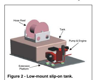
than 100 gallons, the tank width will be just less than the approximate 4 foot wide truck bed. Normally the tank length is around 50 inches. The height varies with the volume of the tank. Figure 3 shows the approximate weight and sizes for typical polypropylene and fiberglass slip-on tanks.
