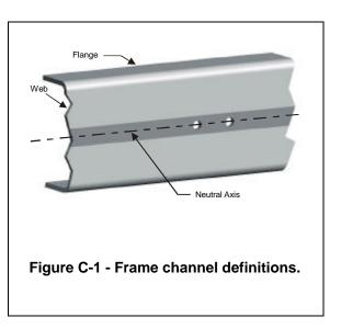
means that the neutral axis is the center line of the frame (halfway down from the top). Figure C-1 illustrates the location of the neutral axis and shows two holes located directly along it. The darker gray stripe illustrates the approximate zone in which it's normally safe to drill.
