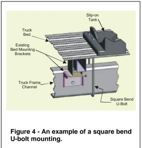
secure the tank against the truck's bed, but not so much that it crushes the frame, bed mounting members or bends the frame's flange.
