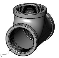
2 NPT Pipe Size, 11 1/2 Threads Per Inch, 0.76" Thread Engagement
